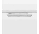
Surface-mounted luminaire with LED, rated life of the LED L90/B50 50000 h (tambient 25°C), colour rendering index CRI > 80, chromaticity tolerance 3 SDCM (initial), wide, homogeneous light distribution pattern (60°), TIR-lens made of PMMA, luminaire housing sheet steel, powder-coated, white, locking mechanism to aligned in 15° steps, rotation angle 300°, In-Track-Adapter, On/Off, 220-240 V~ / 50-60 Hz, max. 27 luminaires per circuit (B16A fuse)
