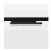
Surface-mounted luminaire with LED, rated life of the LED L90/B50 50000 h (tambient 25°C), colour rendering index CRI > 80, chromaticity tolerance 3 SDCM (initial), wide, homogeneous light distribution pattern (60°), TIR-lens made of PMMA, luminaire housing sheet steel, powder-coated, black, locking mechanism to aligned in 15° steps, rotation angle 300°, In-Track-Adapter, On/Off, 220-240 V~ / 50-60 Hz, max. 27 luminaires per circuit (B16A fuse)
