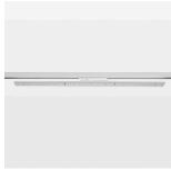
Surface-mounted luminaire with LED, rated life of the LED L90/B50 50000 h (tambient 25°C), colour rendering index CRI > 80, chromaticity tolerance 3 SDCM (initial), wide, homogeneous light distribution pattern (60°), TIR-lens made of PMMA, luminaire housing sheet steel, powder-coated, white, locking mechanism to aligned in 15° steps, rotation angle 300°, In-Track-Adapter, Casambi, On/Off, 220-240 V~ / 50-60 Hz
