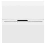
Surface-mounted luminaire with LED, rated life of the LED L90/B50 50000 h (tambient 25°C), colour rendering index CRI > 80, chromaticity tolerance 3 SDCM (initial), wide, homogeneous light distribution pattern (60°), TIR-lens made of PMMA, luminaire housing sheet steel, powder-coated, silver, locking mechanism to aligned in 15° steps, rotation angle 300°, In-Track-Adapter, Casambi, 220-240 V~/50-60 Hz
