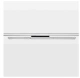
Surface-mounted luminaire with LED, rated life of the LED L90/B50 50000 h (tambient 25°C), colour rendering index CRI > 80, chromaticity tolerance 3 SDCM (initial), double asymmetrical light distribution pattern with slight horizontal brightening, Combination of asymmetrical PMMA lenses and 60 ° TIR lenses made of PMMA, luminaire housing sheet steel, powder-coated, silver, locking mechanism to aligned in 15° steps, rotation angle 300°, In-Track-Adapter, Casambi, 220-240 V~/50-60 Hz
