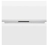
Surface-mounted luminaire with LED, rated life of the LED L90/B50 50000 h (tambient 25°C), colour rendering index CRI > 80, chromaticity tolerance 3 SDCM (initial), double asymmetrical light distribution pattern with horizontal brightening, Combination of asymmetrical PMMA lenses and 30 ° TIR lenses made of PMMA, luminaire housing sheet steel, powder-coated, silver, locking mechanism to aligned in 15° steps, rotation angle 300°, In-Track-Adapter, Casambi, 220-240 V~/50-60 Hz
