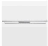
Surface-mounted luminaire with LED, rated life of the LED L90/B50 50000 h (tambient 25°C), colour rendering index CRI > 80, chromaticity tolerance 3 SDCM (initial), extra wide, homogeneous light distribution pattern (90°), TIR-lens made of PMMA, luminaire housing sheet steel, powder-coated, silver, locking mechanism to aligned in 15° steps, rotation angle 300°, In-Track-Adapter, On/Off, 220-240 V~ / 50-60 Hz
