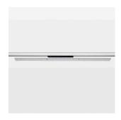
Surface-mounted luminaire with LED, rated life of the LED L90/B50 50000 h (tambient 25°C), colour rendering index CRI > 80, chromaticity tolerance 3 SDCM (initial), double asymmetrical light distribution pattern with slight horizontal brightening, Combination of asymmetrical PMMA lenses and 60 ° TIR lenses made of PMMA, luminaire housing sheet steel, powder-coated, silver, locking mechanism to aligned in 15° steps, rotation angle 300°, In-Track-Adapter, On/Off, 220-240 V~ / 50-60 Hz
