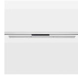
Surface-mounted luminaire with LED, rated life of the LED L90/B50 50000 h (tambient 25°C), colour rendering index CRI > 80, chromaticity tolerance 3 SDCM (initial), double asymmetrical light distribution pattern with slight horizontal brightening, Combination of asymmetrical PMMA lenses and 60 ° TIR lenses made of PMMA, luminaire housing sheet steel, powder-coated, silver, locking mechanism to aligned in 15° steps, rotation angle 300°, In-Track-Adapter, On/Off, 220-240 V~ / 50-60 Hz
