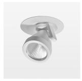
Semi-recessed luminaire with LED, rated life of the LED L80/B10 50000 h (tambient 25°C), colour rendering index CRI > 90, chromaticity tolerance 2 SDCM (initial), reflector with circular light distribution pattern, reflector pure aluminium 99,99% in MIRO-Silver®, segmented and faceted, 3D lens silicon to reduce the proportion of scattered light, die-cast aluminium, powder-coated, rotation angle 400°, swivel angle +/- 85°, white, potentiometer to adjust the brightness, separate driver unit
