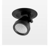
Semi-recessed luminaire with LED, rated life of the LED L80/B10 50000 h (tambient 25°C), colour rendering index CRI > 80, chromaticity tolerance 2 SDCM (initial), reflector with circular light distribution pattern, reflector pure aluminium 99,99% in MIRO-Silver®, segmented and faceted, 3D lens silicon to reduce the proportion of scattered light, die-cast aluminium, powder-coated, rotation angle 400°, swivel angle +/- 85°, black, potentiometer to adjust the brightness, separate driver unit
