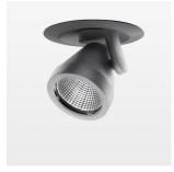
Semi-recessed luminaire with LED, rated life of the LED L80/B10 50000 h (tambient 25°C), colour rendering index CRI > 90, chromaticity tolerance 2 SDCM (initial), reflector with circular light distribution pattern, reflector pure aluminium 99,99% in MIRO-Silver®, segmented and faceted, 3D lens silicon to reduce the proportion of scattered light, die-cast aluminium, powder-coated, rotation angle 400°, swivel angle +/- 85°, silver, potentiometer to adjust the brightness, separate driver unit
