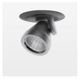
Semi-recessed luminaire with LED, rated life of the LED L80/B10 50000 h (tambient 25°C), colour rendering index CRI > 96, chromaticity tolerance 2 SDCM (initial), reflector with circular light distribution pattern, reflector pure aluminium 99,99% in MIRO-Silver®, segmented and faceted, die-cast aluminium, powder-coated, rotation angle 400°, swivel angle +/- 85°, silver, potentiometer to adjust the brightness, separate driver unit
