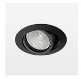
Recessed luminaire with LED, rated life of the LED L80/B10 50000 h (tambient 25°C), colour rendering index CRI > 80, chromaticity tolerance 2 SDCM (initial), reflector with circular light distribution pattern, reflector pure aluminium 99,99% in MIRO-Silver®, segmented and faceted, 3D lens silicon to reduce the proportion of scattered light, die-cast aluminium, powder-coated, rotation angle, swivel angle +/- 25°, black,
