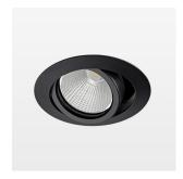
Recessed luminaire with LED, rated life of the LED L80/B10 50000 h (tambient 25°C), colour rendering index CRI > 90, chromaticity tolerance 2 SDCM (initial), reflector with circular light distribution pattern, reflector pure aluminium 99,99% in MIRO-Silver®, segmented and faceted, 3D lens silicon to reduce the proportion of scattered light, die-cast aluminium, powder-coated, rotation angle, swivel angle +/- 25°, black,
