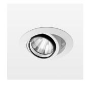
Recessed luminaire with LED, rated life of the LED L80/B10 50000 h (tambient 25°C), colour rendering index CRI > 80, chromaticity tolerance 2 SDCM (initial), rotation-symmetrical reflector with circular light distribution pattern, reflector pure aluminium 99,99% in MIRO-Silver®, segmented and faceted, 3D lens silicon to reduce the proportion of scattered light, die-cast aluminium, powder-coated, rotation angle, swivel angle +/- 25°, white,
