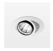
Recessed luminaire with LED, rated life of the LED L80/B10 50000 h (tambient 25°C), colour rendering index CRI > 90, chromaticity tolerance 2 SDCM (initial), rotation-symmetrical reflector with circular light distribution pattern, reflector pure aluminium 99,99% in MIRO-Silver®, segmented and faceted, 3D lens silicon to reduce the proportion of scattered light, die-cast aluminium, powder-coated, rotation angle, swivel angle +/- 25°, white,
