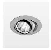
Recessed luminaire with LED, rated life of the LED L80/B10 50000 h (tambient 25°C), colour rendering index CRI > 80, chromaticity tolerance 2 SDCM (initial), rotation-symmetrical reflector with circular light distribution pattern, reflector pure aluminium 99,99% in MIRO-Silver®, segmented and faceted, 3D lens silicon to reduce the proportion of scattered light, die-cast aluminium, powder-coated, rotation angle, swivel angle +/- 25°, silver,
