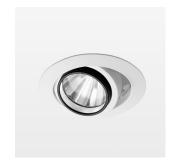
Recessed luminaire with LED, rated life of the LED L80/B10 50000 h (tambient 25°C), colour rendering index CRI > 96, chromaticity tolerance 2 SDCM (initial), rotation-symmetrical reflector with circular light distribution pattern, reflector pure aluminium 99,99% in MIRO-Silver®, segmented and faceted, 3D lens silicon to reduce the proportion of scattered light, die-cast aluminium, powder-coated, rotation angle, swivel angle +/- 25°, white,
