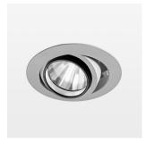
Recessed luminaire with LED, rated life of the LED L80/B10 50000 h (tambient 25°C), colour rendering index CRI > 90, chromaticity tolerance 2 SDCM (initial), rotation-symmetrical reflector with circular light distribution pattern, reflector pure aluminium 99,99% in MIRO-Silver®, segmented and faceted, 3D lens silicon to reduce the proportion of scattered light, die-cast aluminium, powder-coated, rotation angle, swivel angle +/- 25°, silver,
