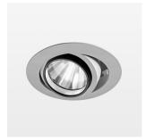
Recessed luminaire with LED, rated life of the LED L80/B10 50000 h (tambient 25°C), colour rendering index CRI > 80, chromaticity tolerance 2 SDCM (initial), rotation-symmetrical reflector with circular light distribution pattern, reflector pure aluminium 99,99% in MIRO-Silver®, segmented and faceted, 3D lens silicon to reduce the proportion of scattered light, die-cast aluminium, powder-coated, rotation angle, swivel angle +/- 25°, silver,
