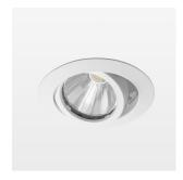
Recessed luminaire with LED, rated life of the LED L80/B10 50000 h (tambient 25°C), colour rendering index CRI > 95, chromaticity tolerance 2 SDCM (initial), rotation-symmetrical reflector with circular light distribution pattern, reflector pure aluminium 99,99% in MIRO-Silver®, segmented and faceted, 3D lens silicon to reduce the proportion of scattered light, die-cast aluminium, powder-coated, rotation angle, swivel angle +/- 25°, white,
