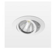
Recessed luminaire with LED, rated life of the LED L80/B10 50000 h (tambient 25°C), colour rendering index CRI > 80, chromaticity tolerance 3 SDCM (initial), rotation-symmetrical reflector with circular light distribution pattern, reflector pure aluminium 99,99% in MIRO-Silver®, segmented and faceted, 3D lens silicon to reduce the proportion of scattered light, die-cast aluminium, powder-coated, rotation angle, swivel angle +/- 25°, white,
