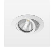
Recessed luminaire with LED, rated life of the LED L80/B10 50000 h (tambient 25°C), colour rendering index CRI > 90, chromaticity tolerance 3 SDCM (initial), rotation-symmetrical reflector with circular light distribution pattern, reflector pure aluminium 99,99% in MIRO-Silver®, segmented and faceted, 3D lens silicon to reduce the proportion of scattered light, die-cast aluminium, powder-coated, rotation angle, swivel angle +/- 25°, white,
