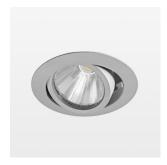
Recessed luminaire with LED, rated life of the LED L80/B10 50000 h (tambient 25°C), colour rendering index CRI > 96, chromaticity tolerance 2 SDCM (initial), rotation-symmetrical reflector with circular light distribution pattern, reflector pure aluminium 99,99% in MIRO-Silver®, segmented and faceted, 3D lens silicon to reduce the proportion of scattered light, die-cast aluminium, powder-coated, rotation angle, swivel angle +/- 25°, silver,
