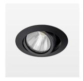
Recessed luminaire with LED, rated life of the LED L80/B10 50000 h (tambient 25°C), colour rendering index CRI > 96, chromaticity tolerance 2 SDCM (initial), rotation-symmetrical reflector with circular light distribution pattern, reflector pure aluminium 99,99% in MIRO-Silver®, segmented and faceted, 3D lens silicon to reduce the proportion of scattered light, die-cast aluminium, powder-coated, rotation angle, swivel angle +/- 25°, black,
