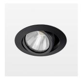
Recessed luminaire with LED, rated life of the LED L80/B10 50000 h (tambient 25°C), colour rendering index CRI > 95, chromaticity tolerance 2 SDCM (initial), rotation-symmetrical reflector with circular light distribution pattern, reflector pure aluminium 99,99% in MIRO-Silver®, segmented and faceted, 3D lens silicon to reduce the proportion of scattered light, die-cast aluminium, powder-coated, rotation angle, swivel angle +/- 25°, black,
