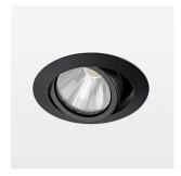
Recessed luminaire with LED, rated life of the LED L80/B10 50000 h (tambient 25°C), colour rendering index CRI > 80, chromaticity tolerance 3 SDCM (initial), rotation-symmetrical reflector with circular light distribution pattern, reflector pure aluminium 99,99% in MIRO-Silver®, segmented and faceted, 3D lens silicon to reduce the proportion of scattered light, die-cast aluminium, powder-coated, rotation angle, swivel angle +/- 25°, black,
