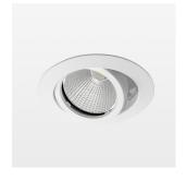
Recessed luminaire with LED, rated life of the LED L80/B10 50000 h (tambient 25°C), colour rendering index CRI > 80, chromaticity tolerance 2 SDCM (initial), reflector with circular light distribution pattern, reflector pure aluminium 99,99% in MIRO-Silver®, segmented and faceted, 3D lens silicon to reduce the proportion of scattered light, die-cast aluminium, powder-coated, rotation angle, swivel angle +/- 25°, white,
