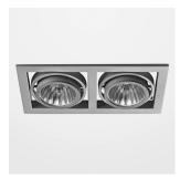
Recessed luminaire with LED, rated life of the LED L80/B10 > 50000 h, colour rendering index CRI > 90, chromaticity tolerance 2 SDCM (initial), reflector with circular light distribution pattern, swivel angle  $\pm$  30° luminaire housing sheet steel, powder-coated, black, separate driver unit
