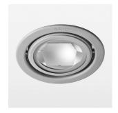
Recessed luminaire with LED, rated life of the LED L80/B10 > 50000 h, colour rendering index CRI > 90, chromaticity tolerance 2 SDCM (initial), reflector with oval light distribution pattern, reflector pure aluminium 99,99% in MIRO-Silver®, swivel angle +/-25°, luminaire housing sheet steel, powder-coated, silver, separate driver unit
