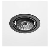
Recessed luminaire with LED, rated life of the LED L80/B10 > 50000h, colour rendering index CRI > 80, chromaticity tolerance 2 SDCM (initial), reflector with circular light distribution pattern, 99,99% pure aluminium, segmented and faceted, cardanic, incl. glass cover, sheet metal powder coated, separate driver unit
