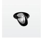
Recessed, flush with ceiling with LED, rated life of the LED L80/B10 > 50000 h, colour rendering index CRI > 82, chromaticity tolerance 2 SDCM (initial), reflector with asymmetrical light distribution pattern, primary reflector and kick reflector 99% pure aluminium in MIRO-Silver®, attachment with kick reflector for light cone projection, exchangeable reflector unit in high-sheen black plastic, with glass cover, luminaire head designed as heat sink die-cast aluminium, black anodized
