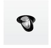
Recessed, flush with ceiling with LED, rated life of the LED L80/B10 > 50000 h, colour rendering index CRI > 95, chromaticity tolerance 2 SDCM (initial), reflector with asymmetrical light distribution pattern, primary reflector and kick reflector 99% pure aluminium in MIRO-Silver®, attachment with kick reflector for light cone projection, exchangeable reflector unit in high-sheen black plastic, with glass cover, luminaire head designed as heat sink die-cast aluminium, black anodized
