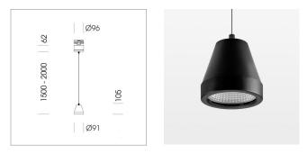
Suspended luminaire with LED, rated life of the LED L80/B10 > 50000 h, colour rendering index CRI > 80, chromaticity tolerance 2 SDCM (initial), reflector with circular light distribution pattern, reflector pure aluminium 99,99% in MIRO-Silver®,segmented and faceted, luminaire head die-cast aluminium, powder-coated, black
