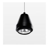
Suspended luminaire with LED, rated life of the LED L80/B10 > 50000 h, colour rendering index CRI > 96, chromaticity tolerance 2 SDCM (initial), reflector with circular light distribution pattern, reflector pure aluminium 99,99% in MIRO-Silver®, segmented and faceted, 3D lens silicon to reduce the proportion of scattered light, luminaire head die-cast aluminium, powdercoated, black
