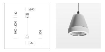
Suspended luminaire with LED, rated life of the LED L80/B10 > 50000 h, colour rendering index CRI > 80, chromaticity tolerance 2 SDCM (initial), reflector with circular light distribution pattern, reflector pure aluminium 99,99% in MIRO-Silver®,segmented and faceted, luminaire head die-cast aluminium, powder-coated, white
