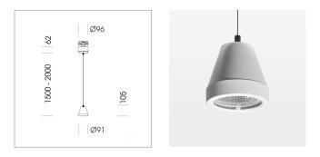
Suspended luminaire with LED, rated life of the LED L80/B10 > 50000 h, colour rendering index CRI > 80, chromaticity tolerance 2 SDCM (initial), reflector with circular light distribution pattern, reflector pure aluminium 99,99% in MIRO-Silver®,segmented and faceted, 3D lens silicon to reduce the proportion of scattered light, luminaire head die-cast aluminium, powder-coated, white
