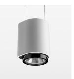
Suspended luminaire with LED, rated life of the LED L80/B10 50000 h (tambient 25°C), colour rendering index CRI > 70, chromaticity tolerance 2 SDCM (initial), reflector with circular light distribution pattern, reflector pure aluminium 99,99% in MIRO-Silver®, segmented and faceted, exchangeable reflector unit in high-sheen black plastic, with glass cover, luminaire housing die-cast aluminium, powder-coated, white Please order canopy and driver unit separatly
