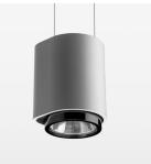
Suspended luminaire with LED, rated life of the LED L80/B10 50000 h (tambient 25°C), colour rendering index CRI > 70, chromaticity tolerance 2 SDCM (initial), reflector with oval light distribution pattern, 3D silicone lens to reduce the proportion of scattered light, reflector pure aluminium 99,99% in MIRO-Silver®, segmented, exchangeable reflector unit in high-sheen black plastic, with glass cover, luminaire housing die-cast aluminium, powder-coated, silver
