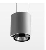
Suspended luminaire with LED, rated life of the LED L80/B10 50000 h (tambient 25°C), colour rendering index CRI > 80, chromaticity tolerance 2 SDCM (initial), reflector with circular light distribution pattern, reflector pure aluminium 99,99% in MIRO-Silver®, segmented and faceted, exchangeable reflector unit in high-sheen black plastic, with glass cover, luminaire housing die-cast aluminium, powder-coated, silver Please order canopy and driver unit separatly
