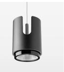
Suspended luminaire with LED, rated life of the LED L80/B10 50000 h (tambient 25°C), colour rendering index CRI > 96, chromaticity tolerance 2 SDCM (initial), reflector with oval light distribution pattern, 3D silicone lens to reduce the proportion of scattered light, reflector pure aluminium 99,99% in MIRO-Silver®, segmented, exchangeable reflector unit in high-sheen black plastic, with glass cover, luminaire housing die-cast aluminium, powder-coated, black
