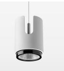
Suspended luminaire with LED, rated life of the LED L80/B10 50000 h (tambient 25°C), colour rendering index CRI > 95, chromaticity tolerance 2 SDCM (initial), reflector with oval light distribution pattern, 3D silicone lens to reduce the proportion of scattered light, reflector pure aluminium 99,99% in MIRO-Silver®, segmented, exchangeable reflector unit in high-sheen black plastic, with glass cover, luminaire housing die-cast aluminium, powder-coated, white
