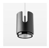
Suspended luminaire with LED, rated life of the LED L80/B10 50000 h (tambient 25°C), colour rendering index CRI > 80, chromaticity tolerance 2 SDCM (initial), reflector with oval light distribution pattern, 3D silicone lens to reduce the proportion of scattered light, reflector pure aluminium 99,99% in MIRO-Silver®, segmented, exchangeable reflector unit in high-sheen black plastic, with glass cover, luminaire housing die-cast aluminium, powdercoated, black
