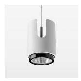
Suspended luminaire with LED, rated life of the LED L80/B10 50000 h (tambient 25°C), colour rendering index CRI > 95, chromaticity tolerance 2 SDCM (initial), reflector with oval light distribution pattern, 3D silicone lens to reduce the proportion of scattered light, reflector pure aluminium 99,99% in MIRO-Silver®, segmented, exchangeable reflector unit in high-sheen black plastic, with glass cover, luminaire housing die-cast aluminium, powdercoated, white
