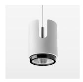
Suspended luminaire with LED, rated life of the LED L80/B10 50000 h (tambient 25°C), colour rendering index CRI > 80, chromaticity tolerance 2 SDCM (initial), reflector with circular light distribution pattern, 3D silicone lens to reduce the proportion of scattered light, reflector pure aluminium 99,99% in MIRO-Silver®, segmented and faceted, exchangeable reflector unit in high-sheen black plastic, with glass cover, luminaire housing die-cast aluminium, powder-coated, white
