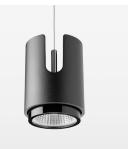
Suspended luminaire with LED, rated life of the LED L80/B10 50000 h (tambient 25°C), colour rendering index CRI > 96, chromaticity tolerance 3 SDCM (initial), reflector with circular light distribution pattern, reflector pure aluminium 99,99% in MIRO-Silver®, segmented and faceted, exchangeable reflector unit in high-sheen black plastic, with glass cover, luminaire housing die-cast aluminium, powder-coated, black Please order canopy and driver unit separatly
