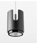
Suspended luminaire with LED, rated life of the LED L80/B10 50000 h (tambient 25°C), colour rendering index CRI > 80, chromaticity tolerance 2 SDCM (initial), reflector with oval light distribution pattern, 3D silicone lens to reduce the proportion of scattered light, reflector pure aluminium 99,99% in MIRO-Silver®, segmented, exchangeable reflector unit in high-sheen black plastic, with glass cover, luminaire housing die-cast aluminium, powder-coated, black
