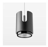
Suspended luminaire with LED, rated life of the LED L80/B10 50000 h (tambient 25°C), colour rendering index CRI > 80, chromaticity tolerance 2 SDCM (initial), reflector with circular light distribution pattern, reflector pure aluminium 99,99% in MIRO-Silver®, segmented and faceted, exchangeable reflector unit in high-sheen black plastic, with glass cover, luminaire housing die-cast aluminium, powder-coated, black
