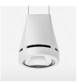
Suspended luminaire with LED, rated life of the LED L80/B10 > 50000 h, colour rendering index CRI > 82, chromaticity tolerance 2 SDCM (initial), reflector with circular light distribution pattern, reflector pure aluminium 99,99% in MIRO-Silver®, luminaire head die-cast aluminium, powder-coated, white, separate driver unit
